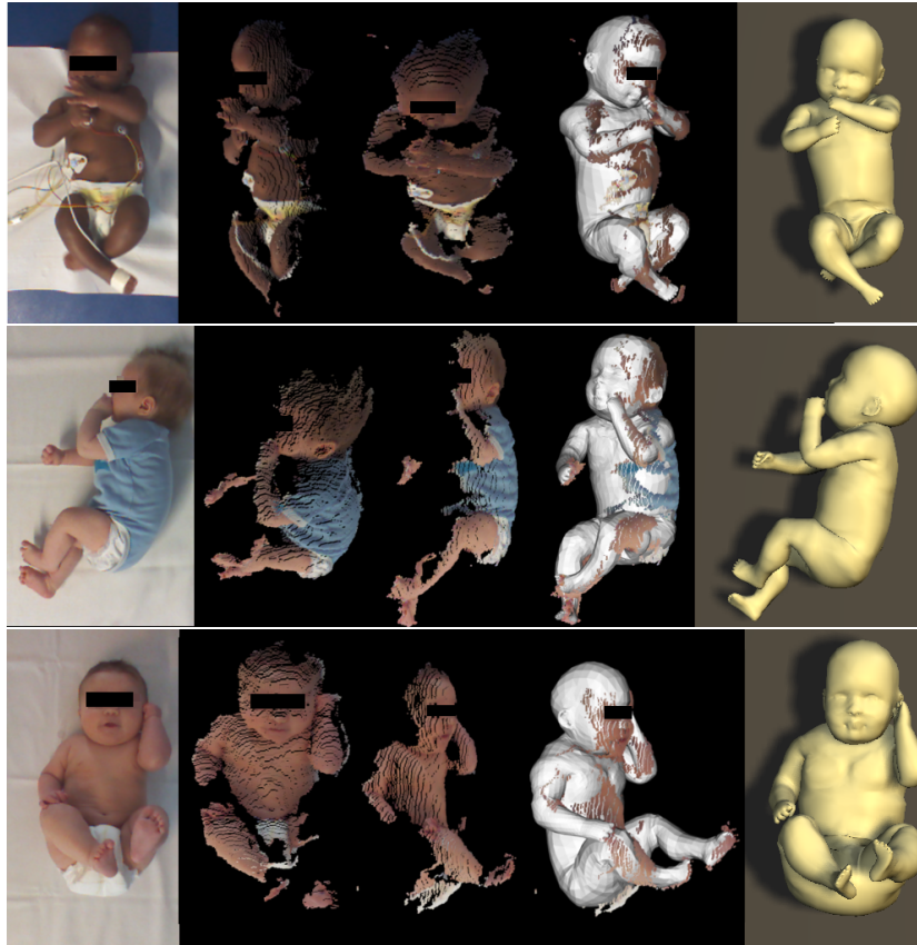
Fig. 6: From left to right: RGB, point cloud, point cloud from other view, point cloud with registered SMIL, rendered registration.
